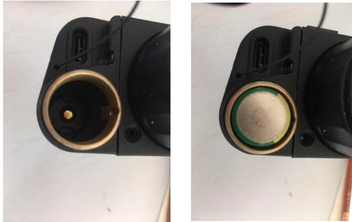
Fig. 5-1 Schematic diagram of battery installation
